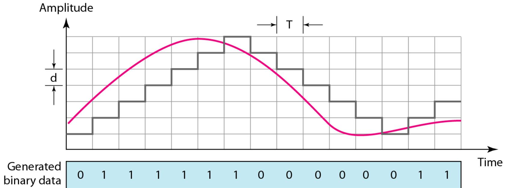
**Figure 4.29** *Delta modulation components*
