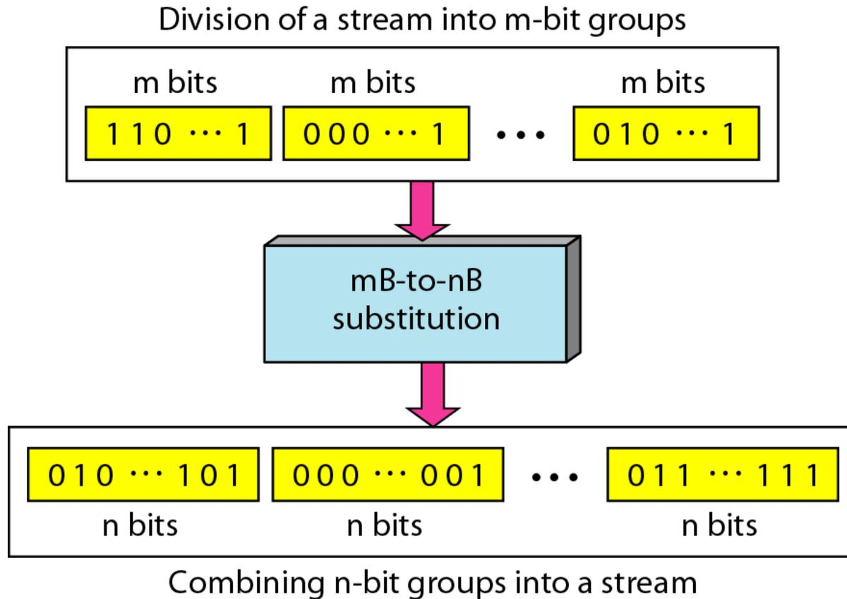
**Figure 4.15** *Using block coding 4B/5B with NRZ-I line coding scheme*
