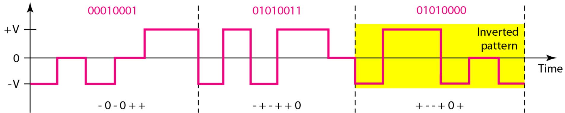
**Figure 4.12** *Multilevel: 4D-PAM5 scheme*
