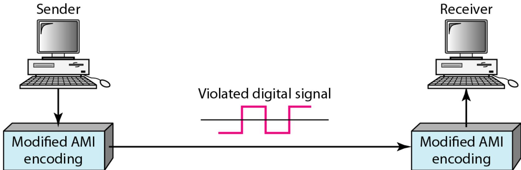
**Figure 4.19** *Two cases of B8ZS scrambling technique*
