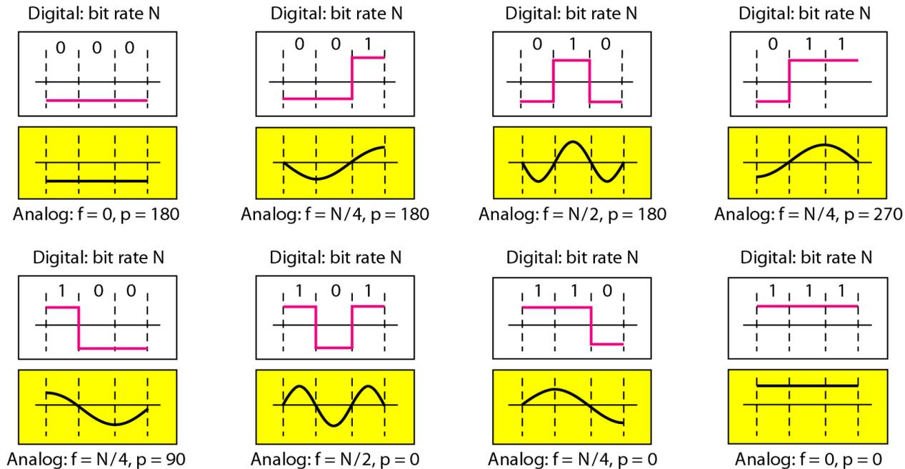
**Figure 3.22** *Simulating a digital signal with first three harmonics*
