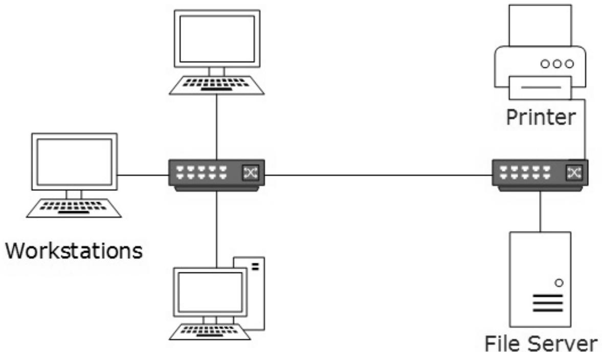
LANs are composed of inexpensive networking and routing equipment. It may contain local servers serving file storage and other locally shared applications. It mostly operates on private IP addresses and does not involve heavy routing. LAN works under its own local domain and is controlled centrally.
