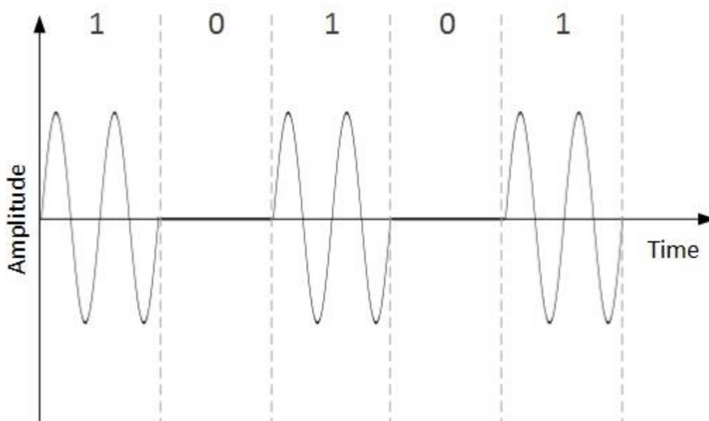
When binary data represents digit 1, the amplitude is held; otherwise it is set to 0. Both frequency and phase remain same as in the original carrier signal.
