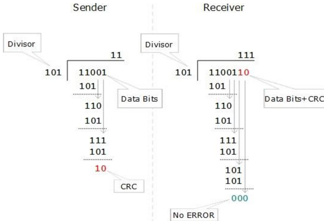
At the other end, the receiver performs division operation on codewords using the same CRC divisor. If the remainder contains all zeros the data bits are accepted, otherwise it is considered as there is some data corruption occurred in transit.
