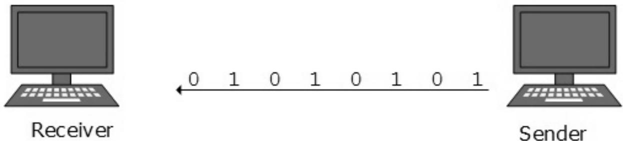
Serial transmission can be either asynchronous or synchronous.
