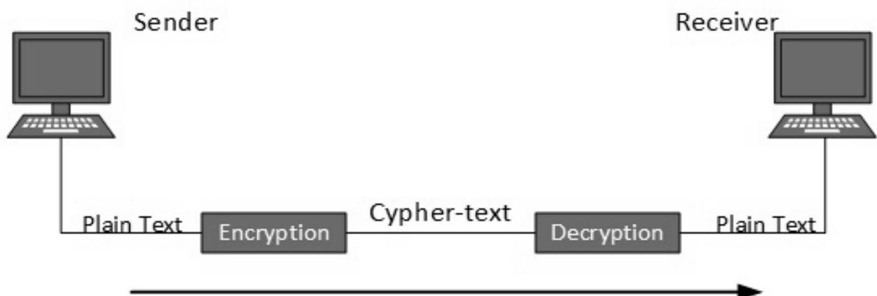
Cryptography is a technique to encrypt the plain-text data which makes it difficult to understand and interpret. There are several cryptographic algorithms available present day as described below:
