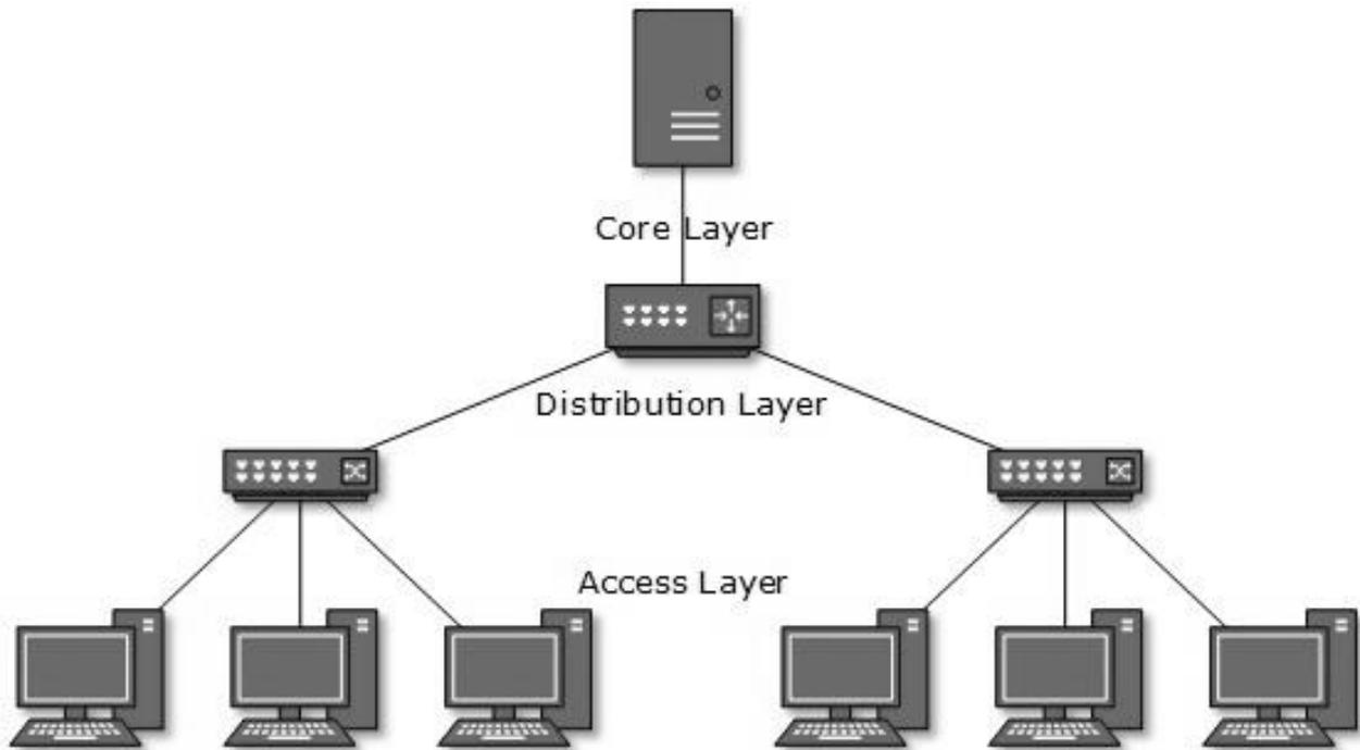
All neighboring hosts have point-to-point connection between them. Similar to the Bus topology, if the root goes down, then the entire network suffers even though it is not the single point of failure. Every connection serves as point of failure, failing of which divides the network into unreachable segment.
