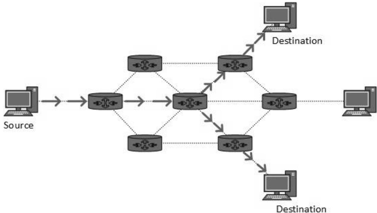
The router must know that there are nodes, which wish to receive multicast packets (or stream) then only it should forward. Multicast routing works spanning tree protocol to avoid looping.
