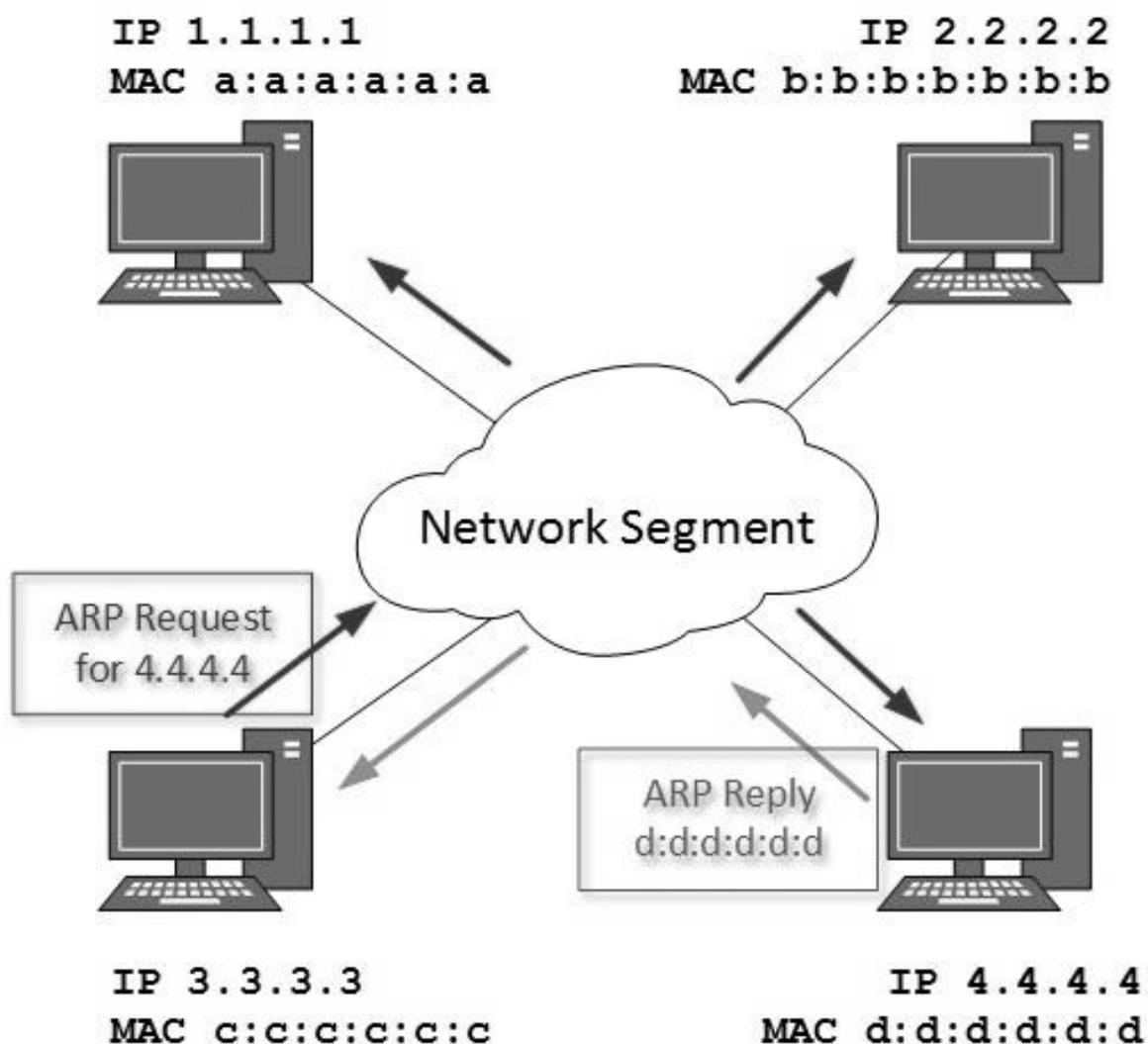
To know the MAC address of remote host on a broadcast domain, a computer wishing to initiate communication sends out an ARP broadcast message asking, "Who has this IP address?" Because it is a broadcast, all hosts on the network segment (broadcast domain) receive this packet and process it. ARP packet contains the IP address of destination host, the sending host wishes to talk to. When a host receives an ARP packet destined to it, it replies back with its own MAC address.
