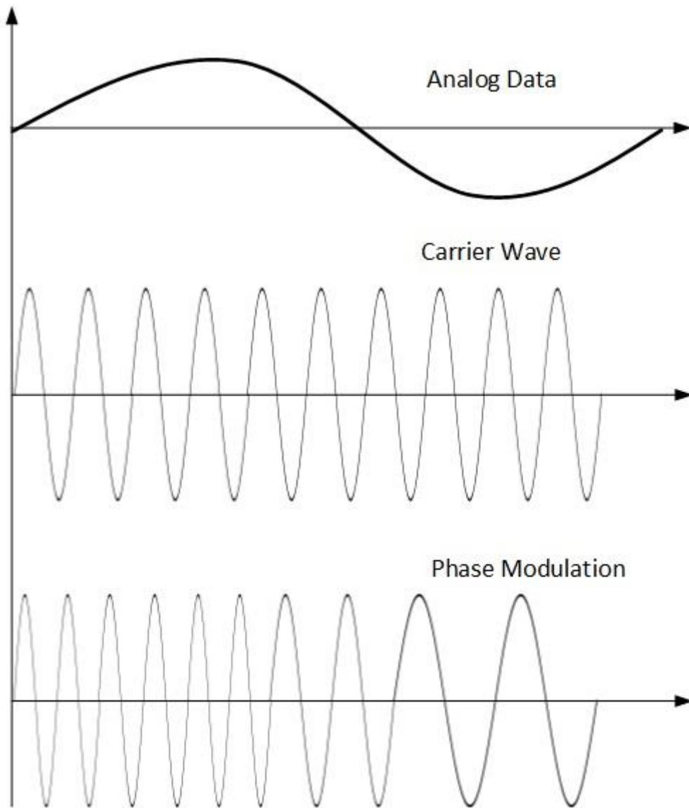
Phase modulation is practically similar to Frequency Modulation, but in Phase modulation frequency of the carrier signal is not increased. Frequency of carrier is signal is changed (made dense and sparse) to reflect voltage change in the amplitude of modulating signal.
