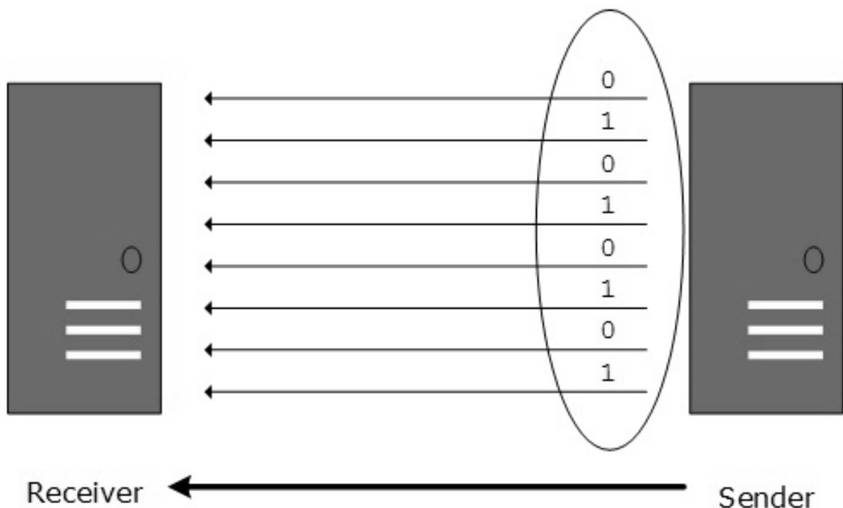
The binary bits are organized into groups of fixed length. Both sender and receiver are connected in parallel with the equal number of data lines. Both computers distinguish between high order and low order data lines. The sender sends all the bits at once on all lines. Because the data lines are equal to the number of bits in a group
