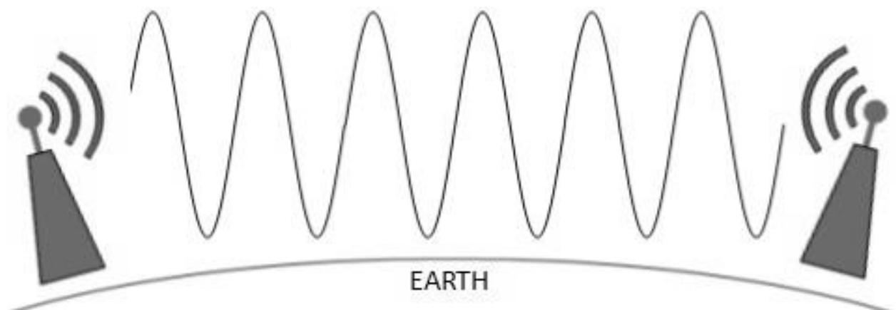
Radio waves of high frequencies are prone to be absorbed by rain and other obstacles. They use Ionosphere of earth atmosphere. High frequency radio waves such as HF and VHF bands are spread upwards. When they reach Ionosphere, they are refracted back to the earth.
