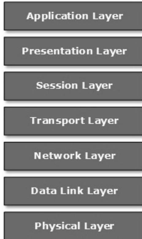
**Application Layer:** This layer is responsible for providing interface to the application user. This layer encompasses protocols which directly interact with the user.
