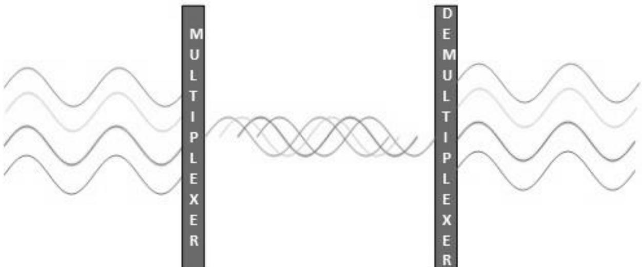
Further, on each wavelength time division multiplexing can be incorporated to accommodate more data signals.
