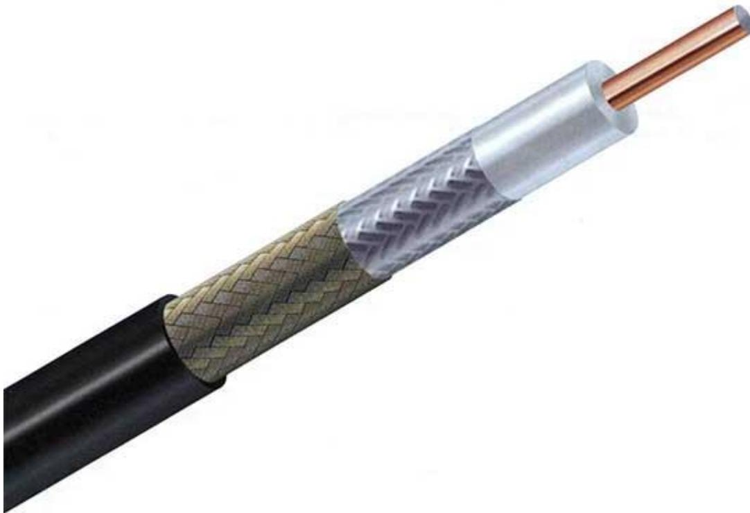
Because of its structure, the coax cable is capable of carrying high frequency signals than that of twisted pair cable. The wrapped structure provides it a good shield against noise and cross talk. Coaxial cables provide high bandwidth rates of up to 450 mbps.
